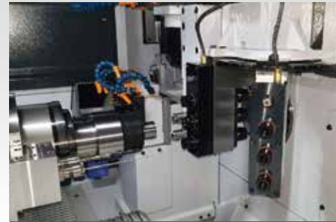
Cross/Face Drilling Function • Cross drilling tool can convert into 3-position face drilling tool for main and sub-spindle. • Able to adjust angle.
