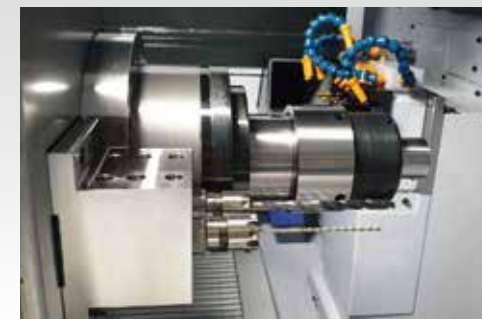
Deep Hole Drilling Device (Max. 135mm) • Sub-spindle can add deep hole drilling device with center coolant function.
